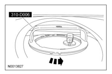
15. NOTICE: The fuel level sensor must be handled carefully to avoid damage to the float arm.
