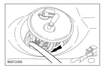
12. **NOTE:** Inspect the surfaces of the <u>FP</u> module flange and fuel tank O-ring seal contact surfaces. Do not polish or adjust the O-ring seal contact area of the fuel tank flange or the fuel tank. Install a new <u>FP</u> module or fuel tank if the O-ring seal contact area is bent, scratched or corroded.
