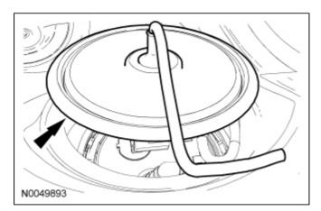
8. **NOTE:** Clean the <u>FP</u> module connections, couplings, flange surfaces and the immediate surrounding area of any dirt or foreign material.
