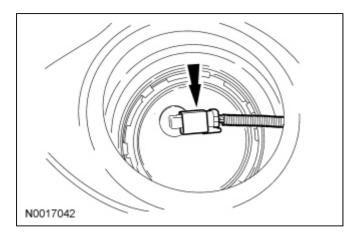
14. *NOTICE:* Carefully install the Fuel Tank Sender Unit Socket to avoid damage to the fuel level sensor when removing the lock ring.
