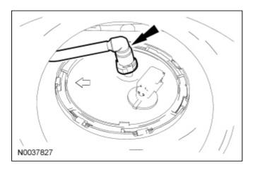
10. NOTICE: Carefully install the Fuel Tank Sender Unit Socket to avoid damage to the Fuel Pump (FP) module when removing the lock ring.
