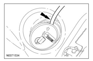
16. **NOTE:** Inspect the surfaces of the fuel level sensor flange and fuel tank O-ring seal contact surfaces. Do not polish or adjust the O-ring seal contact area of the fuel tank flange or the fuel tank. Install a new fuel level sensor or fuel tank if the O-ring seal contact area is bent, scratched or corroded.
