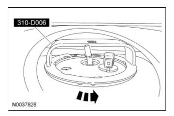
11. NOTICE: The Fuel Pump (FP) module must be handled carefully to avoid damage to the float arm.
